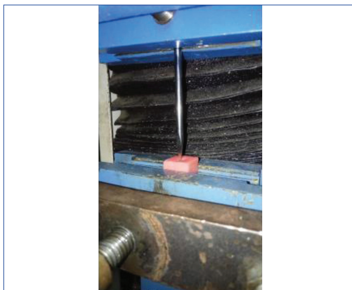
[Table/Fig-3]: Showing sample for testing of compressive strength.
